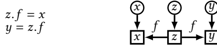
Fig. 7. A minimal program and its (bidirected) SPG. Circles and squares represent variable nodes and object nodes, respectively. Only forward edges are shown.
