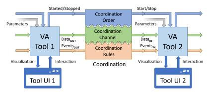
Figure 1: Conceptual abstraction of lightweight coordination between two VA tools. The *coordination order* models any temporal dependency between two tools (i.e., their subsequent or concurrent use). The *coordination channels* capture ways to exchange data between tools, including any necessary data transformations along the way. The *coordination rules* describe automated syncing features between tools as action/reaction pairs.
