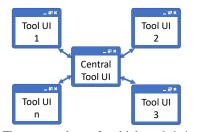
Figure 4: The star topology of multiple tools being used in combination with a central tool UI as mediator.
