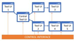
Figure 5: The control interface that serves as a global parametrization facility and for displaying process information. In this context VA tools can be utilized as a combination of single (UI 1 and UI 3), pair-wise (UI 4 and UI 5), and multiple (UI 2) references from a central hub application (Central UI).
