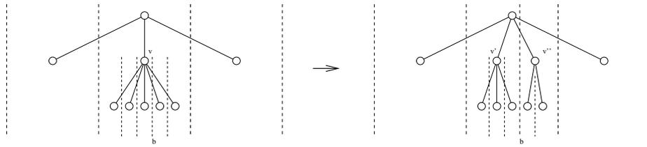
**Fig. 12.** Splitting a node;  $v$  splits along  $b$ , which becomes a new boundary in  $\text{parent}(v)$ .
