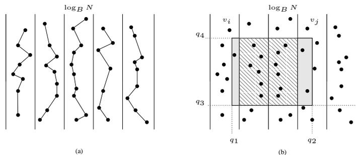
**Fig. 17.** a) The slabs corresponding to a node  $v$  in the base tree and the segments projected onto the  $y$ -axis and stored in an interval tree. (b) A query  $q = (q_1, q_2, q_3, q_4)$  is naturally decomposed into a part in  $X_{v_i}$ , a part in  $X_{v_j}$ , and a part that spans all slabs  $X_{v_k}$  for  $i < k < j$ .
