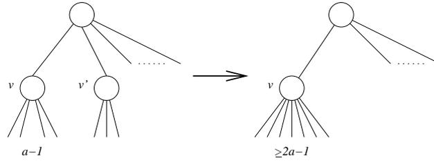
**Fig. 4.** Fusing degree  $a - 1$  node  $v$  (or leaf with  $a - 1$  elements) with sibling  $v'$ .
