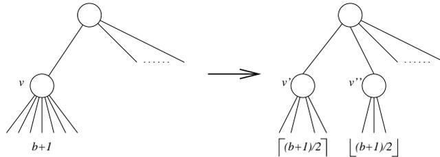
**Fig. 3.** Splitting degree  $b + 1$  node  $v$  (or leaf with  $b + 1$  elements) into nodes  $v'$  and  $v''$ .
