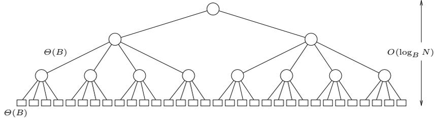
**Fig. 2.** B-tree. All internal nodes (except possibly the root) have fan-out  $\Theta(B)$  and there are  $\Theta(N/B)$  leaves. The tree has height  $O(\log_B N)$ .
