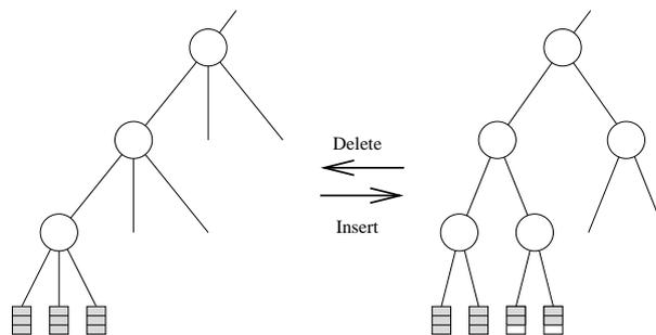
**Fig. 5.** Alternating insertion and deletion of the same element in an  $(2,3)$ -tree can cause  $\Theta(\log_a N)$  rebalancing operations each.
