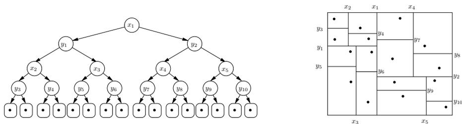
**Fig. 19.** A kd-tree and the corresponding partitioning.
